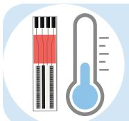
5. When storing sensors for over a year, keep them in a refrigerator. When storing them for less than one year, keep them at a temperature of less than 20° C.
