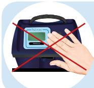
3. Do not disturb the instrument or sample during the test.
